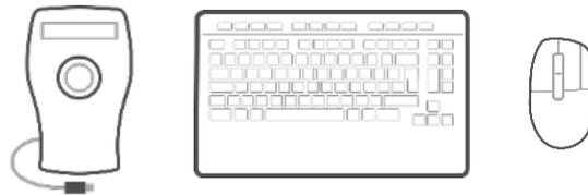
Place the SpaceMouse Enterprise on the opposite side of the keyboard to your standard mouse. One hand engages the 3D mouse to position your model: rotating, panning and zooming. The other hand uses the standard mouse to select, create and edit.
